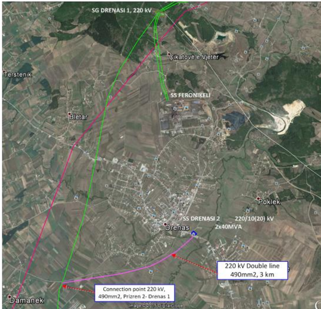
Figure 5-21. Satellite imagery of SS Drenas 2 and the layout of the dual 220kV
