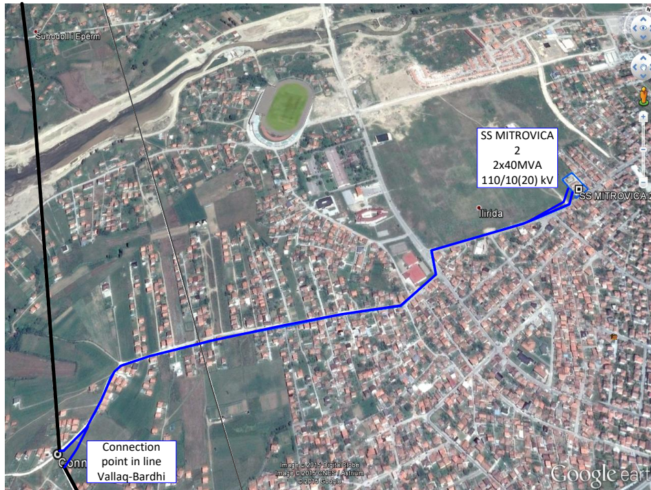
Figure 5-13 Satellite view of the location of SS Mitrovica 2 and dual cable path to the point of connection
