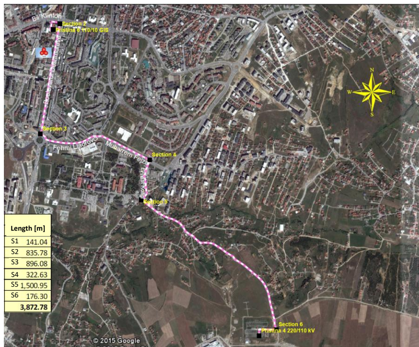
Figure 5-14. Geographical position of two SS Prishtina 4 and Dardania and the proposed route of the 110 kV double cable line
